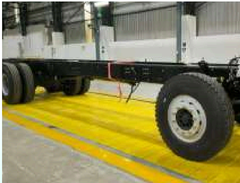
Chasis Pre-Assembly on Chain Conveyor
